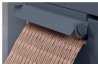
Creation of padding mats (one layer of cardboard, HSM ProfiPack P425).
