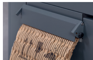
Creation of compressed packaging material with a closed compression flap (two layers of cardboard, HSM ProfiPack P425).
